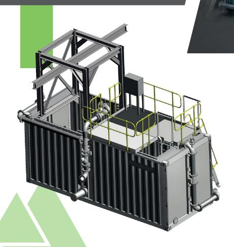
With a capacity of 32000 Litres our test facility allows us to test both Submersible and End Suction Centrifugal Pumps up to a maximum Kilowatt Rating of 132kW in various Voltages, namely 380/415V, 525/550V as well as 1000V depending on the available Voltage on each specific site.
