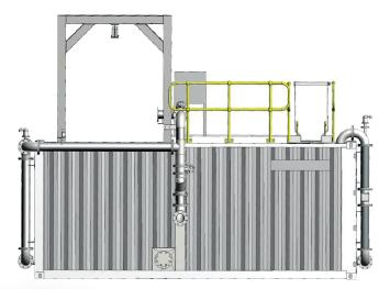
Electrical Actuated Control Valves regulates the pressure to allow a pump test to be done at different pressure positions on the pump curve while the flow meter measures the corresponding flow at these specific points. This allows a pump test curve to be plotted and compared to the OEM curve to ensure the pump repair has been done according to OEM standards.
